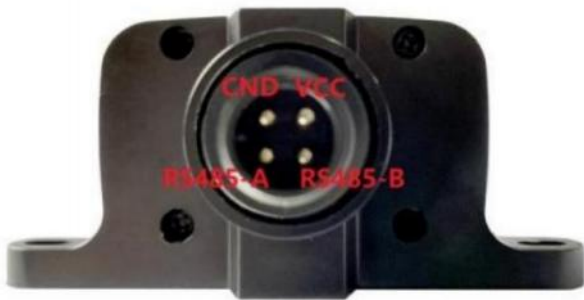
Definition of 4G/Wifi module's aviation plug-in interface
